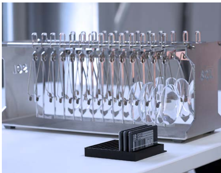
Fig. 4: Example for batch coating process. Picture: Satisloh
