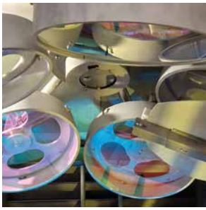
Planetary with customizable substrate holder design
