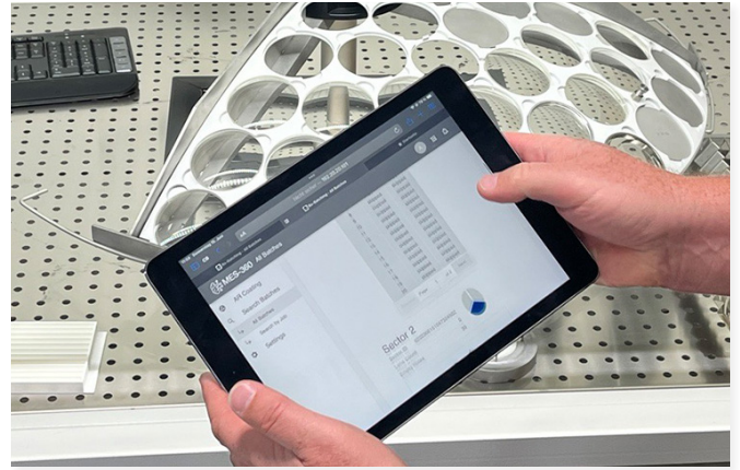
MES-360 Coating Batch, tracks lenses during the coating process
